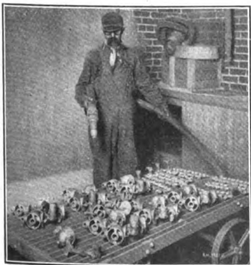
FIG. 7. SAND BLASTING CARBURETER CASTINGS
