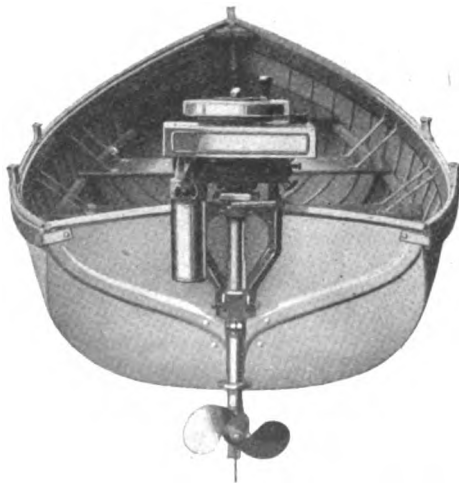
REAR VIEW OF MULLINS STEEL BOAT MADE EXPRESSLY FOR OUTBOARD MOTORS. NOTE WIDE STERN.
